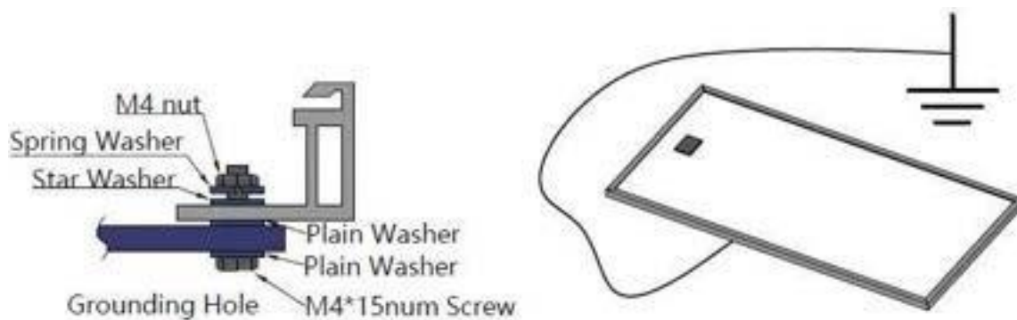
Figure 7: Ground installation of PV modules
